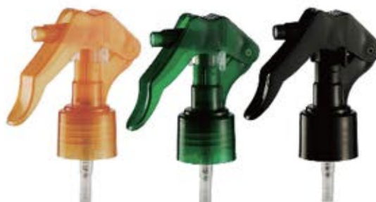
专利号: PAT.No. ZL 2003 3 0108192.0 TS-031 型喷头 剂量 0.25ml & 0.75ml TS-031 0.25ml & 0.75ml 600PCS/CTN meas.: 45X39X40cm DIA: Ø22/410 Ø24/410
