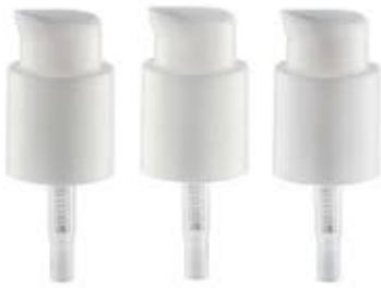
5#-E-0.5ml 液体分配器 PUMP 5#-E, Output: 0.5ml 1250 PCS/CTN, Meas.: 45x39x46cm DIA: Ø22mm
